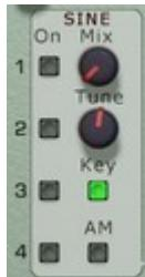
The Sine Wave oscillator can be used to reinforce the fundamental or sub-octave of a voice.
